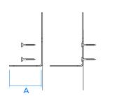
For cavity barriers 77mm-90mm wide (across cavity) use 2 MP brackets and the 65mm long spike (A).
