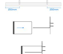
Fix 2 number MP brackets, per linear meter, to the substrate at maximum 250mm from the end of the cavity barrier, with a maximum spacing between brackets of 500mm.
