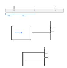
Fix 3 number MP brackets, per linear meter, to the substrate at maximum 150mm from the end of the cavity barrier, with a maximum spacing between brackets of 350mm.
