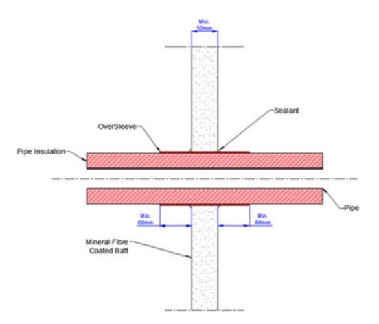
Copper, Steel & Cast Iron Insulated Pipes Or other pipes of class A1 in accordance with EN 13501-1 with a melting or decomposition point higher than the nominal furnace temperature at the intended classification time (e.g. 1049°C at 120 minutes)
