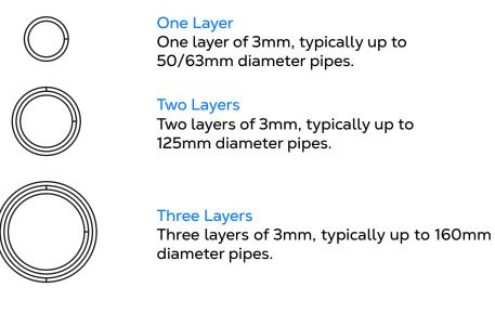
NB. For larger pipe diameters which require >1000mm length of OverSleeve, the length can be made up of more than length of OverSleeve and the join sealed with the supplied glass scrim reinforced repair tape, minimum 200mm length of repair tape.
