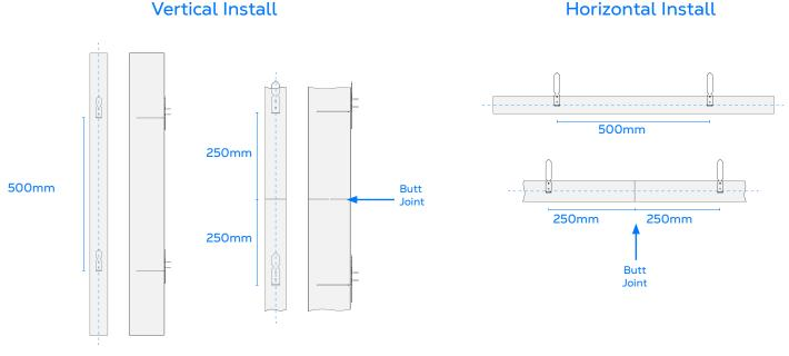
Push the cavity barrier onto the bracket spike, the brackets should impale the NVFB to approximately mid barrier depth and must not protrude through the face of the cavity barrier, remembering to allow for the final compression against the outer substrate also. The cavity barrier should be pushed fully onto the bracket spike and sit flush with the substrate, at the rear of the cavity barrier, ensuring that there are no gaps behind the cavity barrier.
