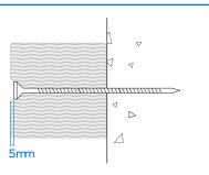
Use stainless steel screws, with a maximum head diameter of 12.5mm and with a length suitable for the cavity barrier and the substrate. Ensure that the screw head fully penetrates the face of the cavity barrier, the screw head should sit at least 5mm behind the face of the cavity barrier. Care should be taken not to compress the surface more than 10mm as this may effect the performance of the cavity barrier.
