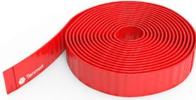
Tenmat's CavGuard Roll 65 is a cavity fire barrier designed to firestop the cavity behind external walls consisting of outer substrates of masonry or brickwork. The low smoke zero halogen highly expansive intumescent material allows ventilation to be maintained in non-fire conditions.
