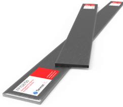
Tenmat's FF102/50, Ventilated Cavity Fire Barriers, are manufactured from a low smoke zero halogen high expansion intumescent material. They are designed to reinstate fire resisting performance to external wall cavities that are required to be ventilated (open-state) in non-fire conditions.
