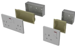
Tenmat's Socket Box Inserts, are manufactured from halogen free, low smoke, fire resistant, mineral fibre material and are designed to maintain the fire performance of partition (stud) wall constructions when penetrated by steel or plastic electrical back boxes. The insert will also provide resistance to the passage of sound and air movement.
