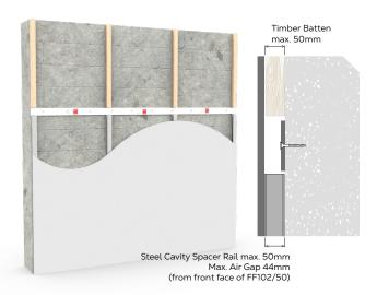
Tested detail includes for various non-combustible outer substrates including mineral fibre external wall slab (full details can be provided upon request).
