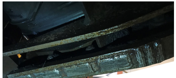
Ferobide in photo welded to AR400 steel, in good shape after 4 months
