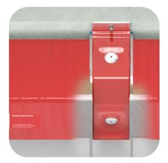
Ensure the profile of the cut VFB Plus allows tight fitting either side of the support bracket and allows a continuous intumescent seal formed by the VFB Plus and CavGuard MSC.
