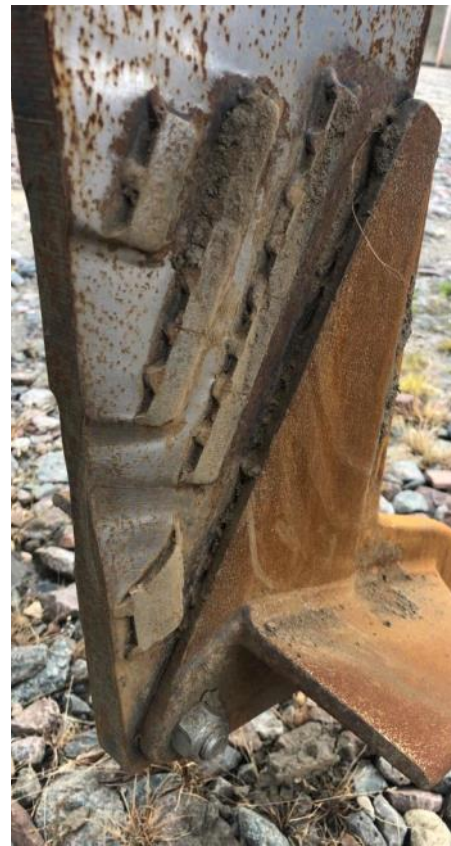
Ferobide tiles applied to the legs have effectively prevented wearing of the base metal during 3 years and counting with no additional maintenance required.
