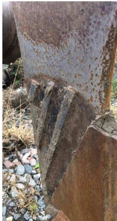
Ferobide tiles applied to the legs have effectively prevented wearing of the base metal during 3 years and counting with no additional maintenance required.
