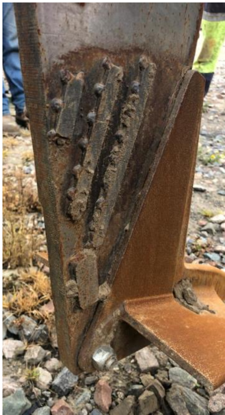
Ferobide tiles applied to the legs have effectively prevented wearing of the base metal during 3 years and counting with no additional maintenance required.
