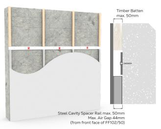
When stopping and starting vertical timber battens, ensure a gap of min. 10 mm is left above and below the FF102/50
