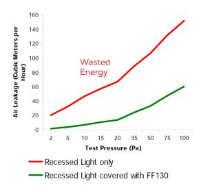
When downlights penetrate a loft space, then they can allow moisture ladened air to enter the loft space which can cause premature rotting of roof timbers, Tenmat FF130 loft covers meet the full requirements of the NHBC vapour transmission by minimising the passage of water vapour.
