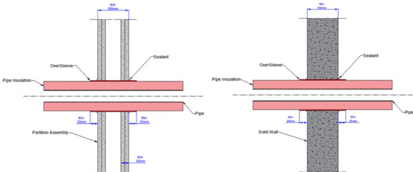
Copper, Steel & Cast Iron Insulated Pipes
