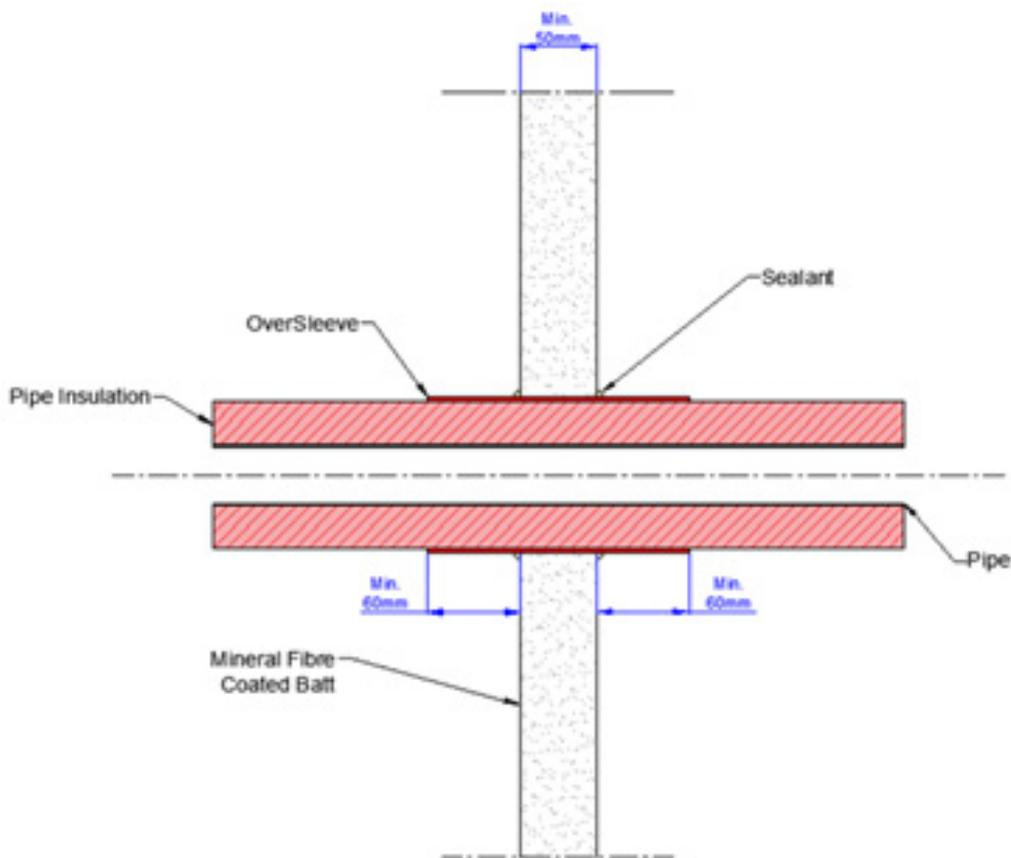
Copper, Steel & Cast Iron Insulated Pipes
