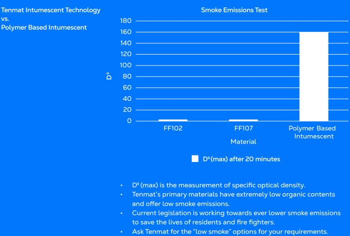
• Low Smoke - Exova Lab Tested according to BS EN45545-2
