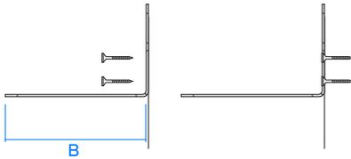
For cavity barriers 216mm-275mm wide (across cavity) use 3 MP brackets and the 160mm (B) long spike. To secure the bracket use nom. 5mm Ø stainless steel screws/fixings, with a maximum head diameter of 13mm and with a length and type suitable for the substrate.
