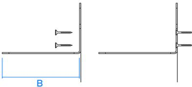
For cavity barriers 91mm–215mm wide (across cavity) use 2 MP brackets and the 160mm (B) long spike. To secure the bracket use nom. 5mm Ø stainless steel screws/fixings, with a maximum head diameter of 13mm and with a length and type suitable for the substrate.
