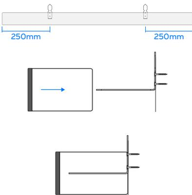
For cavity barriers 91mm–215mm wide (across cavity) use 2 MP brackets and the 160mm long spike. The 160mm spike will require cutting to size, if used in barriers less than 185mm wide, to ensure that the spike does not pierce through the face of the intumescent material, the bracket should be cut to provide a minimum projection through the barrier to 3/4 of the cavity barrier width and to a maximum of 25mm behind the face of the intumescent strip.
