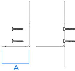
For cavity barriers 76mm-90mm wide (across cavity) use 2 MP brackets and the 65mm (A) long spike.
