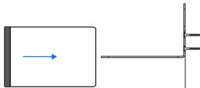
Where sections of cavity barrier are less than 1 linear meter in length, ensure that MP brackets are positioned at a maximum 150mm from each end.
