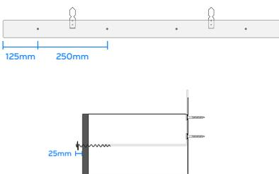
Screw the pigtail screws through the face of the intumescent material on the face of the cavity barrier (the face with the labels).
