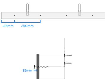
Screw the pigtail screws through the face of the intumescent material on the face of the cavity barrier (the face with the label).
