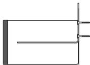
The cavity barrier should be pushed fully onto the bracket spike and sit flush with the substrate, at the rear of the cavity barrier, ensuring that there are no gaps behind the cavity barrier.
