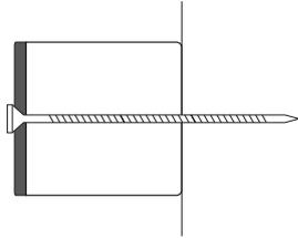
Use stainless steel countersunk head screws, with a maximum head diameter of 16mm and with a length suitable for the size of cavity barrier and sufficient fixing depth into the substrate.
