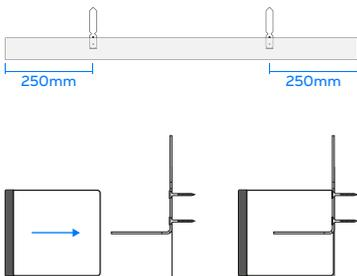
Fix 2 number MP brackets, per linear meter, to the substrate at maximum 250mm from the end of the cavity barrier, with a maximum spacing between brackets of 500mm.
