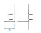
For cavity barriers 76mm-90mm wide (across cavity) use 2 MP brackets and the 65mm (A) long spike.
