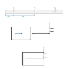
Fix 3 number MP brackets, per linear meter, to the substrate at maximum 150mm from the end of the cavity barrier, with a maximum spacing between brackets of 350mm.
