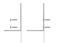
Where sections of cavity barrier are less than 1 linear meter in length, ensure that MP brackets are positioned at a maximum 250mm from each end.
