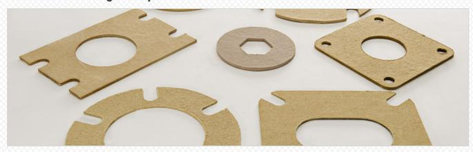
**TENMAT** *FIREFLY* FF 700 has been specially developed as a commercial grade of millboard that is both strong and flexible with very low shrinkage at 1000°C. It provides outstanding performance as a universal gasketing, heat shield, and insulation material.
