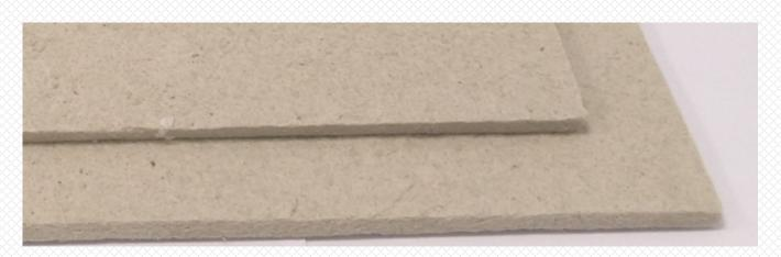
TENMAT FIREFLY FLEX FFF1000 has been specially developed as a commercial grade of flexible millboard that is both strong and flexible with very low shrinkage at 1000 °C. It provides outstanding thermal performance as a universal gasketing, heat shield, and insulation material.
