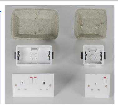
The **TENMAT** *FIREFLY* 109 Socket Box covers are designed to be installed behind both single and double recessed switch/socked boxes. In a fire situation, the cover expands internally to fill all of the available space with a fire resistant highly insulating char. The fire is unable to penetrate the hole and the cover is able to give additional insulation protection to the wall void by reducing the chance of fire damage to flammable structural members.
