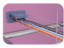
Once cables have been installed they should be tightly sealed with **TENMAT** Infill Material
