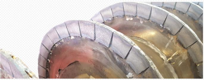
Decanter centrifuge fitted with Ferobide tiles
