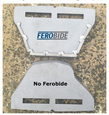
Once tack welded in place, fully weld Ferobide tiles along back edge.
