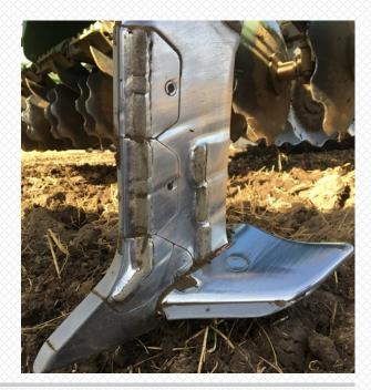
The point below would typically complete 250 acres on a 5metre cultivator before wearing out. After applying Ferobide behind the tungsten in 3 rows this point has already completed 650 acres.
