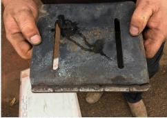
"This subsoiler was fitted with these scrapers and has since completed over 3000 acres of abrasive sand land. There has been a saving of £1500 worth of wearing metal, 60 man hours maintenance, with an outlay of only £225."
