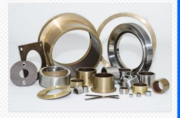
**TENMAT** FEROGLIDE bearings are used extensively by valve manufacturers due to the material's ability to maintain low friction under heavy loads. FEROGLIDE bearings have a metal backing and a composite self lubricating liner. This gives a combination of high strength, excellent chemical resistance, and low coefficient of friction which means that FEROGLIDE is the material of choice for oil and gas valves in both sub-sea and platform applications.
