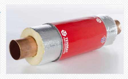
The **TENMAT** *FIREFLY* OverSleeve is a universal, one-product-fits-all solution for the firestopping of insulated metal pipes. The thin and flexible intumescent is quickly and simply wrapped directly on top of pipe insulation without the need to cut back, ensuring that thermal and vapour seal performance is maintained. The red branded foil can be easily checked and identified on site to confirm that firestopping is in place.
