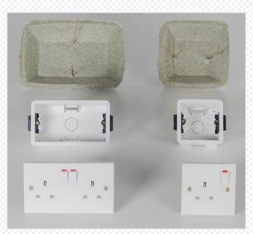
The **TENMAT** *FIREFLY* 109 Socket Box Covers are designed to be installed behind both single and double recessed switch/socket boxes. In a fire situation, the cover expands internally to fill all of the available space with a fire resistant highly insulating char. The fire is unable to penetrate the hole and the cover is able to give additional insulation protection to the wall void by reducing the chance of fire damage to flammable structural members.
