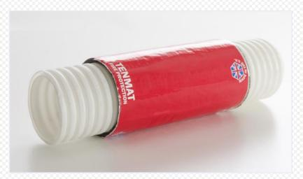
The **TENMAT** *FIREFLY* OverSleeve is a universal, one-product-fits-all solution for the firestopping of cable bundles and cable conduits. The thin and flexible intumescent is quickly and simply wrapped directly onto the conduit. The red branded foil can be easily checked and identified on site to confirm that firestopping is in place.
